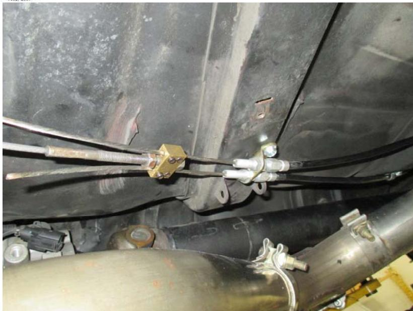
The next issue was to adapt the new parking brake to the existing parking pedal cable. We ordered Wilwood's universal parking brake kit which included cables from the emergency brake levers on each rear brake and a brass adapter to capture the two cables and combine them to the existing parking brake cable. This all went in under the GTO and looks great while working just like the old emergency brake did.
